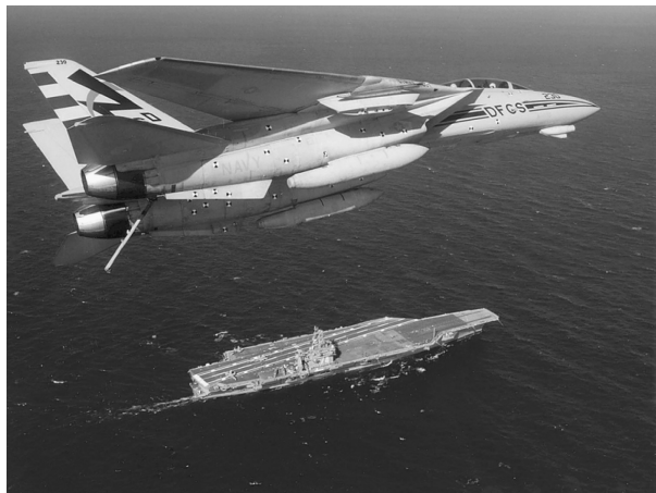
Fig. 16 F-14 does not exhibit wing-rock tendencies at transonic conditions.
